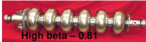
Superconducting 805 MHz multi-cell cavities of SNS linac. V = 10-15 MV, DF = 6\% .
