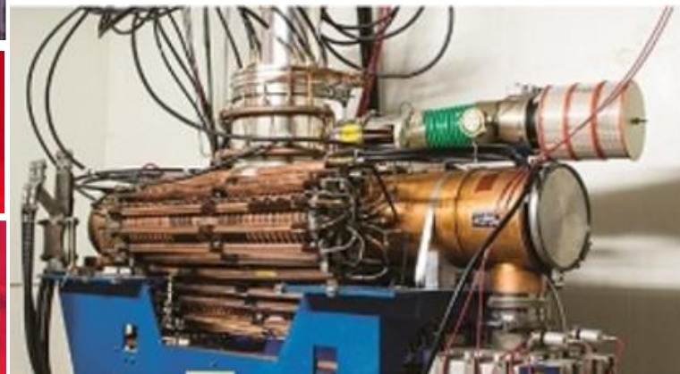
Tunable cavity for FNAL Booster Synchrotron F = 37.8-52.8 MHz. V = 60 kV, DF = 50\%
