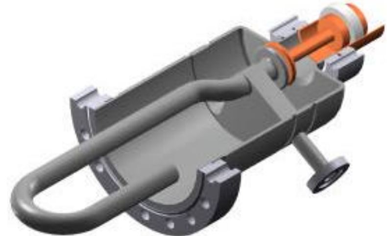
LHC HOM coupler, Q_{ext} < 200 for most “dangerous” modes
